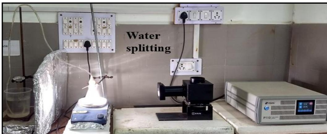
**Figure 2.8** Instrumentation of the water splitting during experimental.
