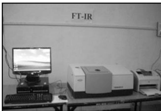
**Figure 2.2 Bruker -Tensor FT-IR Spectrophotometer**
