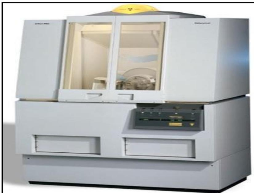
**Figure 2.1** PANalytical system diffractometer (Model: *XPERT-3*)
